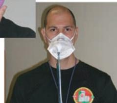
The quantitative fit test actually measures the level of protection using the TSI PortaCount. The quantitative fit test determines a fit factor by measuring and comparing concentrations of a challenge agent inside and outside the respirator.
